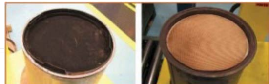
The photo on the left shows a diesel particulate filter prior to cleaning. The one on the right shows what a cleaned DPF should look like.
